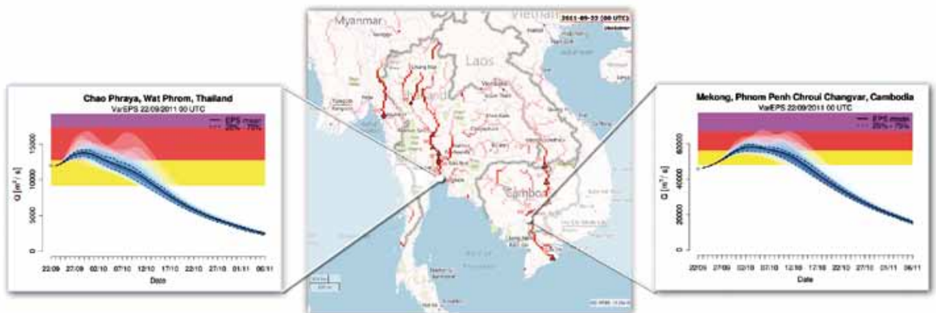
Figure 18: GloFAS 45-day probabilistic discharge forecasts for the Chao Phraya (Thailand) and the lower Mekong (Cambodia) on 22 September 2011
