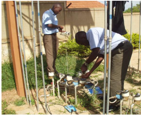
In situ small meter testing with meters in series.
