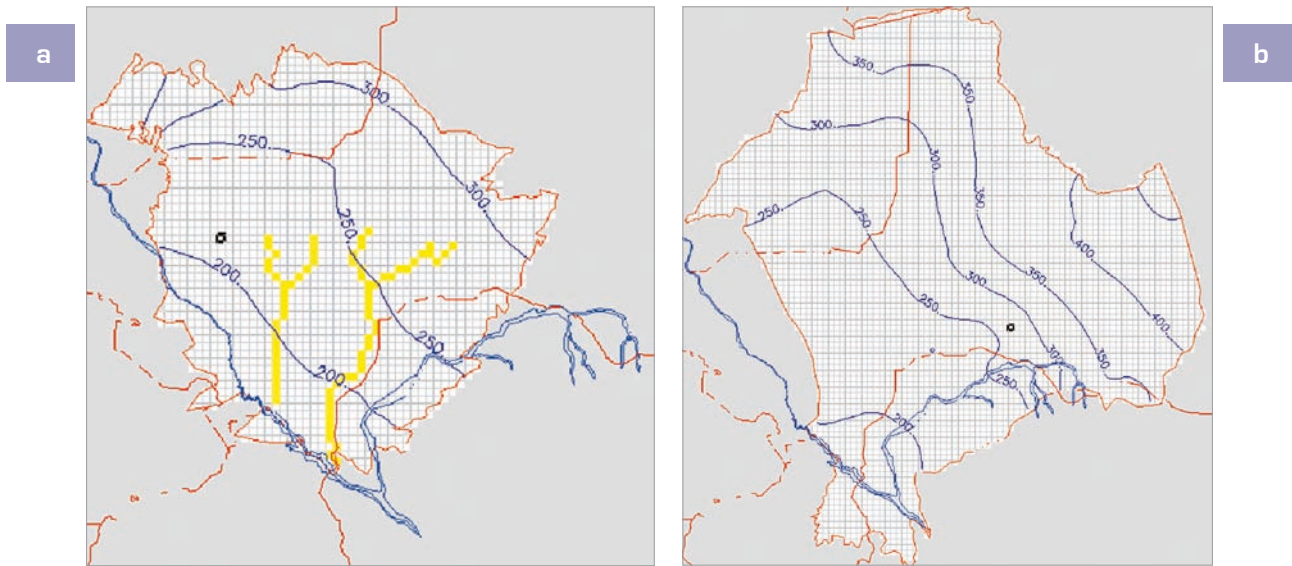
FIGURE 44 : The CT(a) and the Ci(b) piezometric maps calculated by the model in 2004
