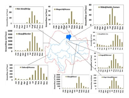
Figure 5. Streamflow at different gauging stations
