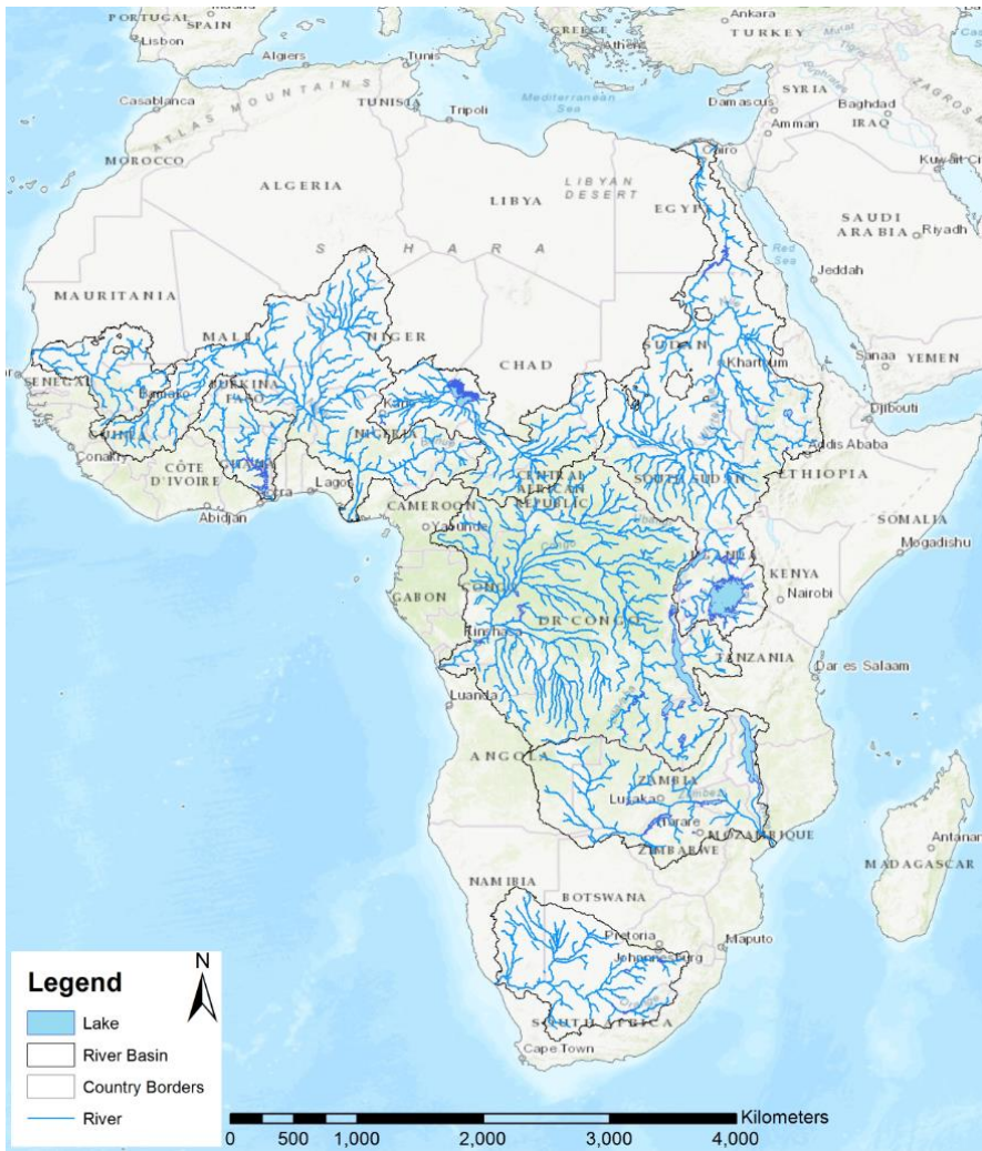
Figure 4 - River network and surface water, i.e. lakes and wetlands, as resulting from the analysis of the Digital Elevation Data (Beck et al., 2014; Lehner and Döll, 2004; Lehner and Grill, 2011) (Figure from Farinosi et al., 2017b).
