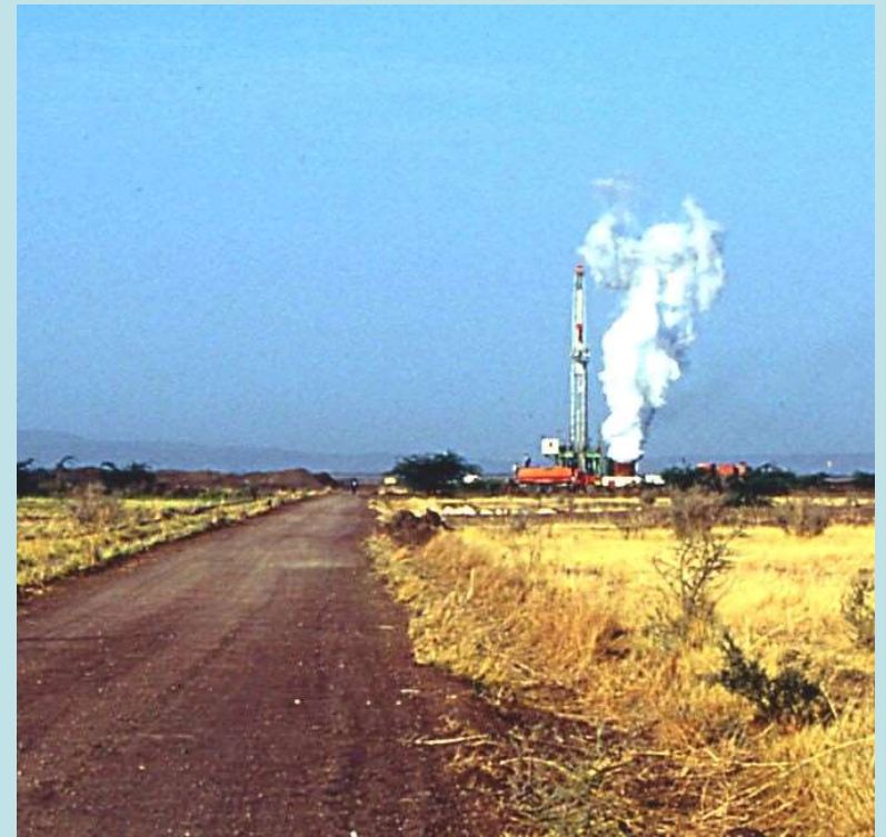
(TD-4 production tests at Dubti Geothermal Field (1995), Tendaho Rift, Afar Region - Ethiopia)
