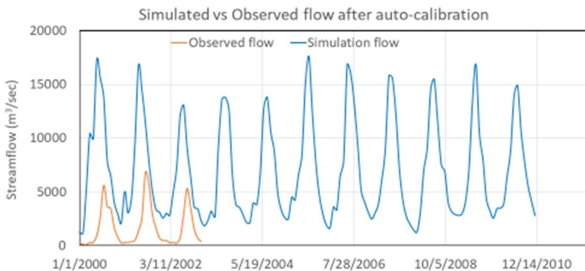
Figure. The simulated and observed streamflow is not matching even after auto-calibrating MIKE-NAM rainfall-runoff model at GERD.
