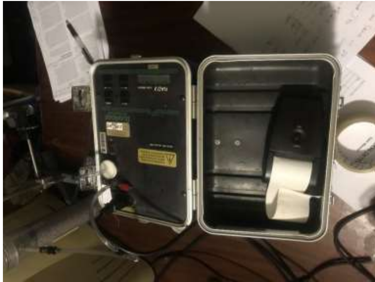
Figure 1. RAD 7 Radon Detector.
