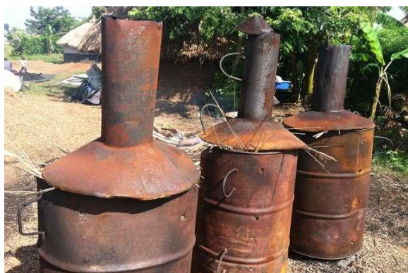
Figure 2. Example of slow pyrolysis units: on the left, small unit employed in Uganda (Paing, 2015); on the right, large unit employed in Senegal (Pro-natura, 2017).
