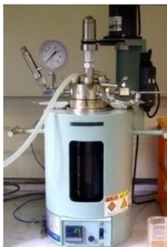
Figure 3. Example of a HTC pilot unit (Riu Lohri et al., 2013).
